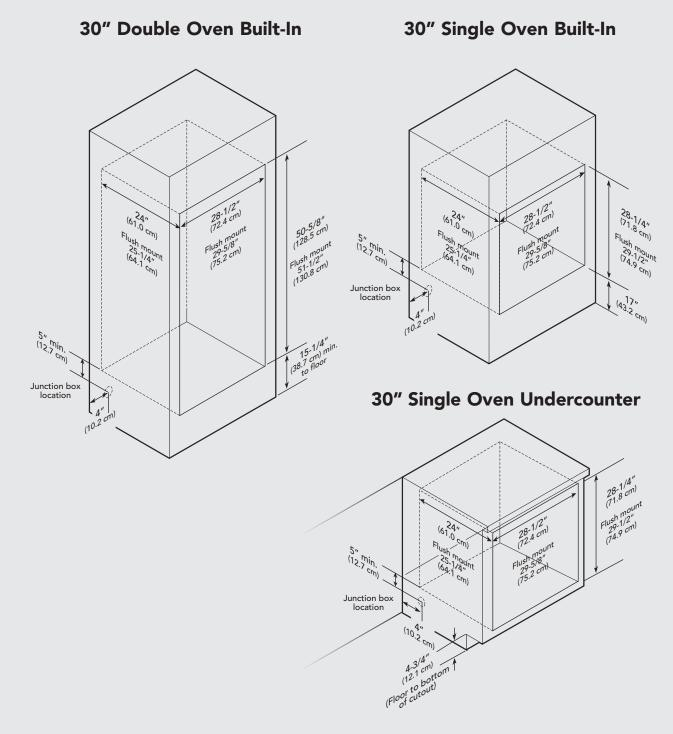
\*Note: To install the oven in a flush mount application the flush mount accessory kit (D30FTS for single ovens and D30FTD for double ovens) is required.
