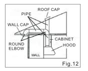
a. Decide the location and measure the length of venting pipe from the hood to the outside. (Fig.12)
