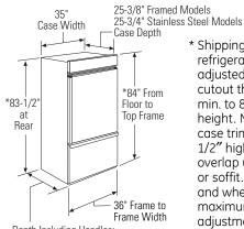
\* Shipping height. The refrigerator can be adjusted to fit into a cutout that is 83-1/2" min. to 84-1/2" max. height. Note that the top case trim at the front is 1/2" higher and will overlap upper cabinetry or soffit. Use leveling leas and wheels for a maximum 1" height adjustment.
