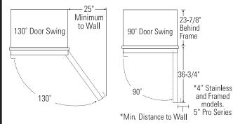
Allow 25" minimum clearance for a full 130° door swing. Allow 15" for pan removal.
