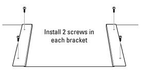
• Install the "L" brackets onto each side of the cutout. The wide flat portion should be on top of the opening. Install 2 screws into the top of each bracket.
