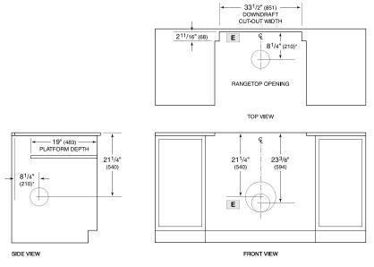
$<sup>^{\</sup>star}6"$  (152) back from countertop cut-out when internal blower is rear mounted.
