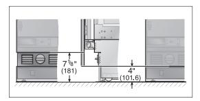
If required by the surrounding cabinetry design, the distance between the bottom edge of the door panel and the floor can be increased from approx. 4" (102 mm) up to 7 1/8" (181 mm), but should not be decreased. Note, however, that the venting grille and (if applicable) water filter cavity will be visible, even if the door is closed.
