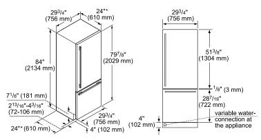
\*Excludes thickness of door panel. If standard panel with 3/4" thickness is mounted, total depth is 24 3/4".
