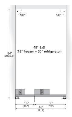
**IMPORTANT:** Just as with standalone columns, always ensure that the receptacles and the water line are correctly positioned. For dimensional requirements see page 234.
