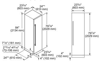
\*Excludes thickness of door panel. If standard panel with 3/4" thickness is mounted, total depth is 24 3/4".
