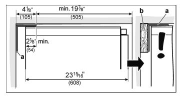
The length of the plank should correspond to the width of the installation enclosure!
