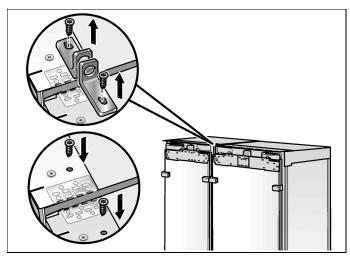
To attach the cover strip to the attachment plate (top):
