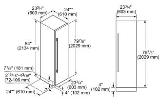
\*Excludes thickness of door panel. If standard panel with <sup>3</sup>/4" thickness is mounted, total depth is 24 <sup>3</sup>/4".
