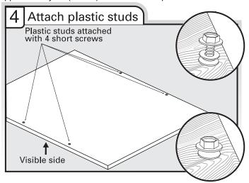
Attach the 4 plastic studs to the wooden panel using the four  $\frac{5}{6}$ " hex-head (short) screws provided.
