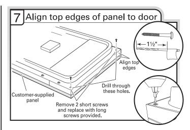
Open the door and align top edges. Use tape to mark a 32 drill bit to gauge the hole depth of approximately 12 (3.8 cm). Drill pilot holes into the top corners of the door, using hole in liner as a guide.
