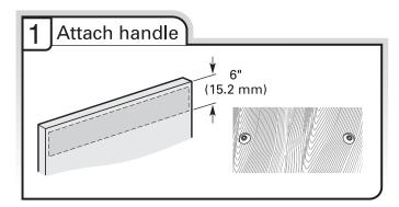
Install the custom hardware handle(s) on the front of the wooden panel inside dotted line.
