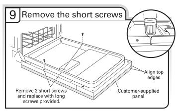
Remove the short screws (3rd from top) on either side of the inner door panel. Use tape to mark a  $\frac{3}{2}$  drill bit to gauge the hole depth of approximately  $1\frac{1}{2}$  (3.8 cm). Drill 2 pilot holes using the door liner hole as a guide into the panel. Install the 2 remaining long screws.
