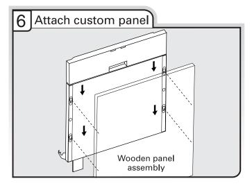
Align the studs on the custom wood panel to the keyhole slots on the door assembly. Ensure that all 4 plastic studs are engaged in the keyhole slots. Slide wood panel down until the top surface of the wooden panel is flush with the top of the door.
