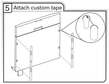
Check custom tape alignment with metal door slots; verify tape is right-side up, and that the tape does not overhang the metal door on the top, bottom or side interfaces. Remove the backing from the custom tape by pulling straight down on the liner. Align the custom tape to the keyhole slots on the metal door (see "5 Attach custom tape) and apply. Repeat steps for one side and then the other.
