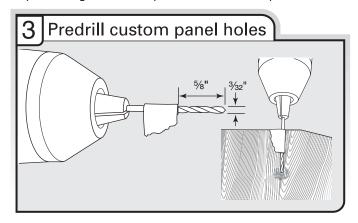
**NOTE:** Do not drill deeper then %" (16 mm) to keep from drilling through panel. Pilot hole depths given are for %" (19 mm) thick panel.
