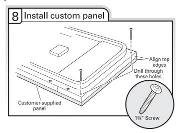
Using a Torx® T15® screwdriver, install two #8 x 1%" screws in top corners to secure custom wood panel in place.
