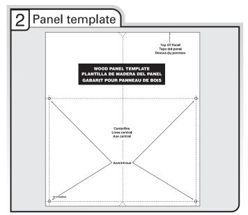
Using the template provided, attach it to the backside of the custom panel with tape. Make sure that the center of the template is aligned with the center of the wooden panel and top of the template is aligned to the top face of the wooden panel.
