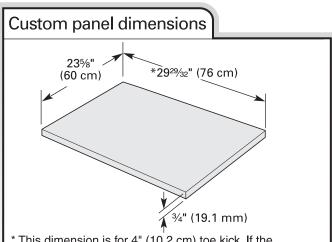
\* This dimension is for 4" (10.2 cm) toe kick. If the installation needs a higher toe kick, adjust the height of the wood panel accordingly except on models with fan assisted dry. Fan models have a duct at the bottom of the door that would be exposed if shorten the door panel for toe kick heights above 4" (10.2 cm). Toe kick heights greater than 6" (15.2 cm) are not recommended for this product.
